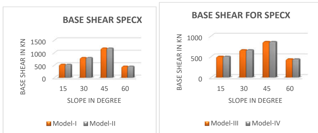
Tab: Fig.22:Base shear in the X direction for models I and II
