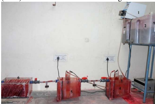
Fig. 1: Experimental setup used in the study (1= Peristaltic Pump; 2= Overhead Tank; 3=DC Power Supply Unit; 4= Reactor 1; 5= reactor 2; 6= Lamella Settler)
