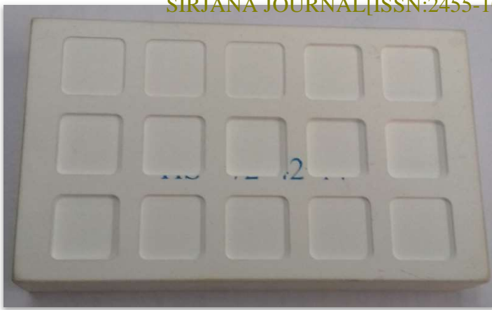
Fig. 1. (a) Zirconia Ceramic work piece; (b) TiAlN coated tool (Titanium Aluminium Nitride).
