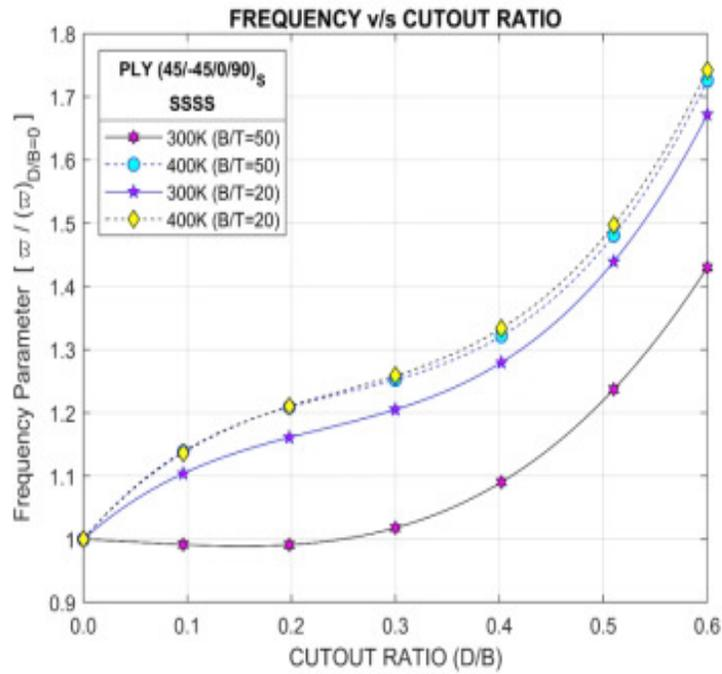
**Figure 5.** Influence of temperature and thickness ratio on vibration for cutout panels with simply supported boundary condition.
