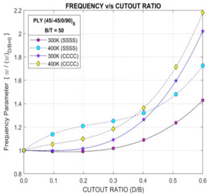
**Figure 6.** Influence of temperature and boundary condition on vibration for cutout panels with thickness ratio (B/T) 50.
