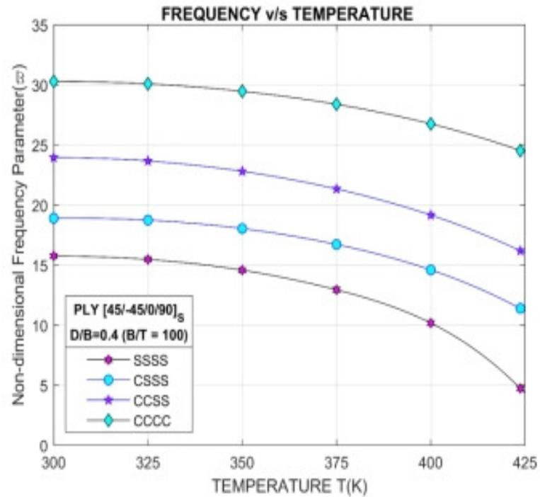
**Figure 4.** Variation in frequency as a function of temperature T (K) for the centrally located circular cutout panel (D/B=0.4) and thickness ratio (B/T=100) for various boundary condition
