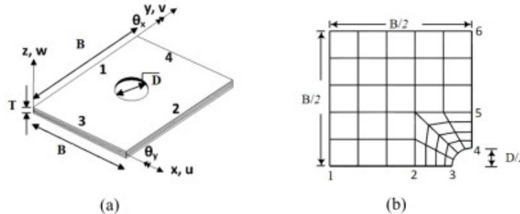
**Figure 2.** (a) Geometry of the Laminated panel (b) Mesh pattern of cutout panel.
