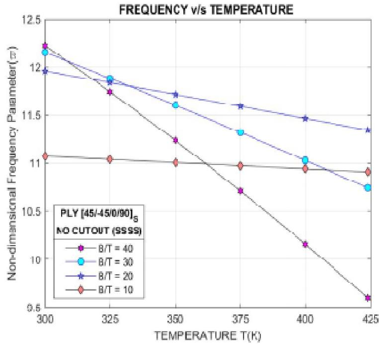
**Figure 3.** The effect of plate thickness on the frequency of a simply supported plate composed of (45/-45/0/90)<sub>S</sub> laminate, subjected to temperature variations without any cutout, is under investigation.
