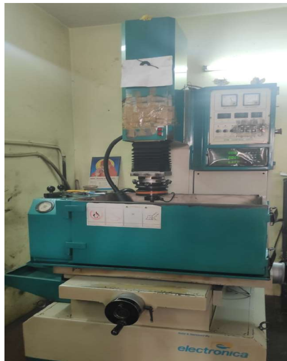
Fig.3 Experimental set up of EDM process
