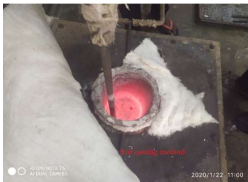
Fig: 1 Stir Casting Method
