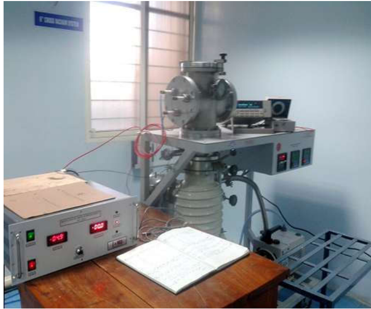
Figure 2: Custom designed FE measurement system fixture inside the Vacuum chamber.
